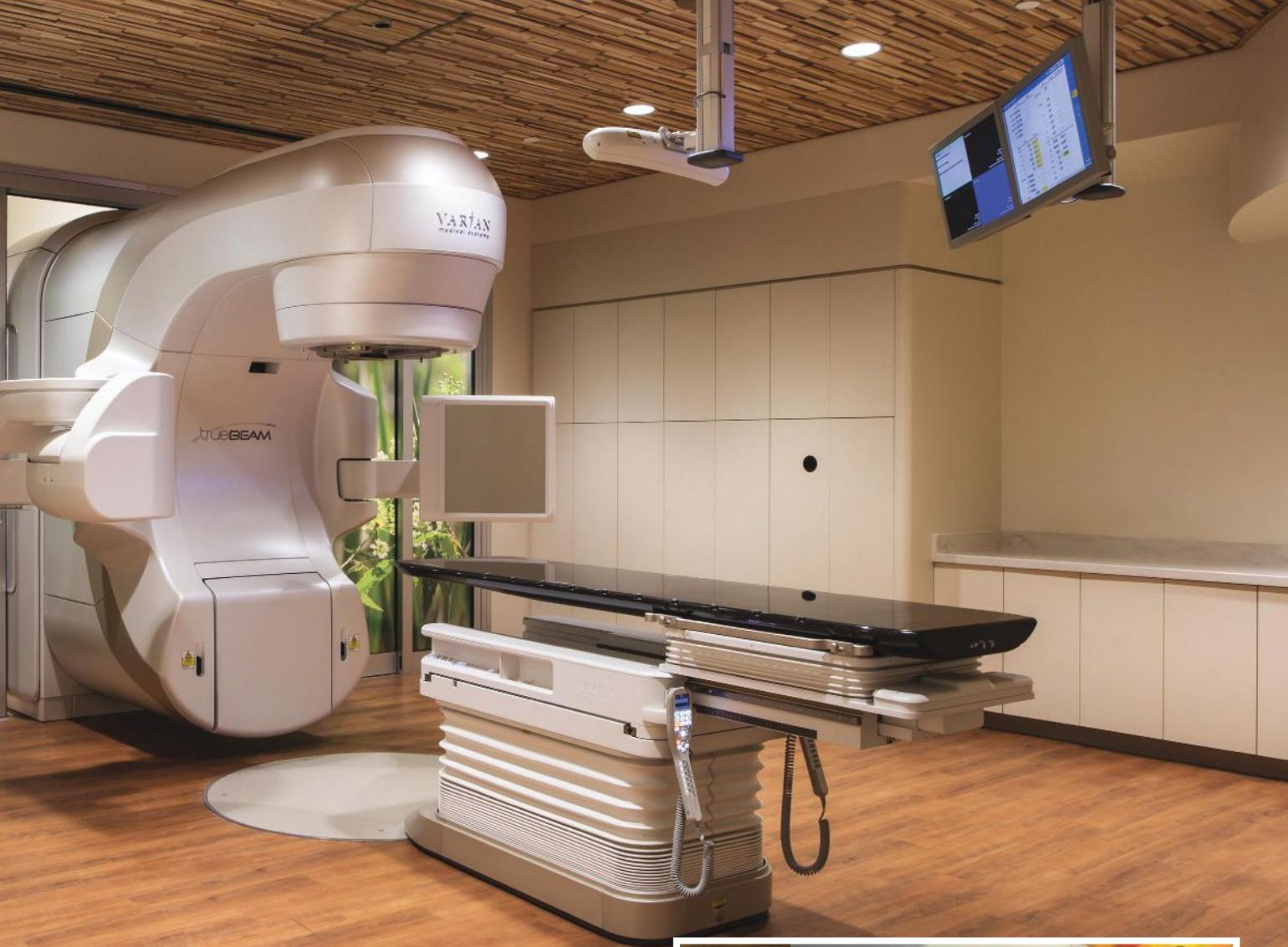
Site prep and replacement of a new linear accelerator for the Providence Del Amo Diagnostic Center included a new vault door as well as structural, mechanical, electrical and plumbing upgrades.
